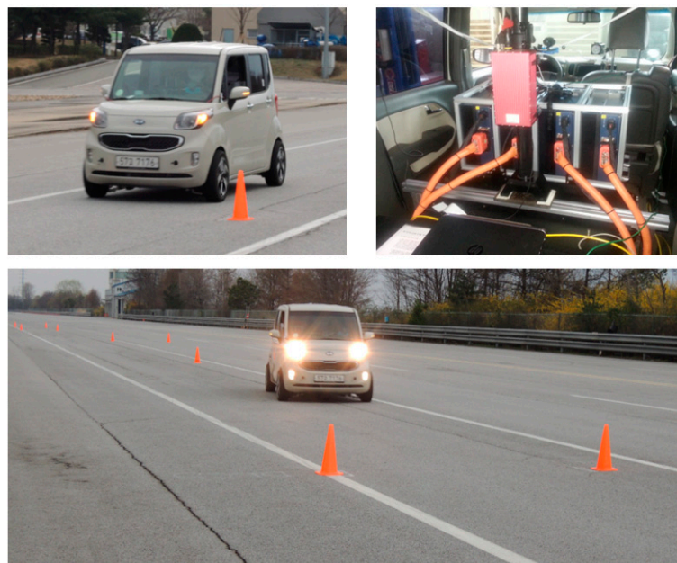
Figure 17. Slalom test and measuring sensor.
